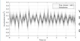
Vehicle acceleration time history Solid line: experiment average Gray area:  $\pm$  1-3 standard deviation Dashed line: simulation result
